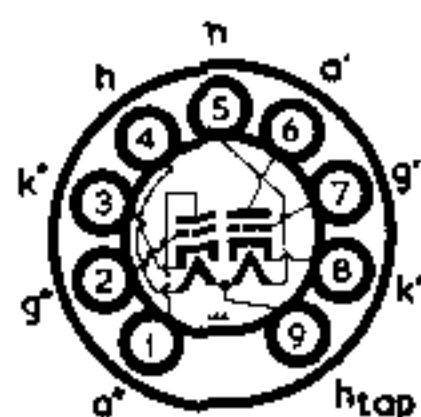
The BRIMAR 6067 is a trustworthy miniature double triode (Low-mu) with separate cathode connections and a tapped heater enabling it to be used in a variety of applications.
